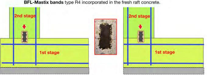
The BFL-Mastix bands type R4 are tightly anchored in both, raft and wall conrete.
