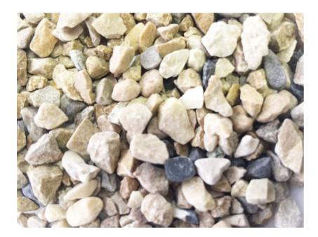
Even with a minimum of cement paste in the concrete, the angular form of the gravel aggregates assures a perfect liaison in the concrete, even avoiding an enrichment of the cement quantity in the concrete.
