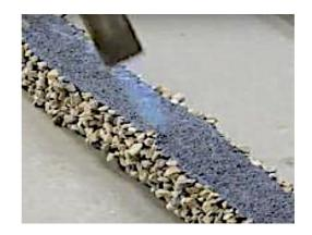
To control the adherence of a glued waterstop with Mastix MS-Polymer, it just needs trying to pull off the band.
