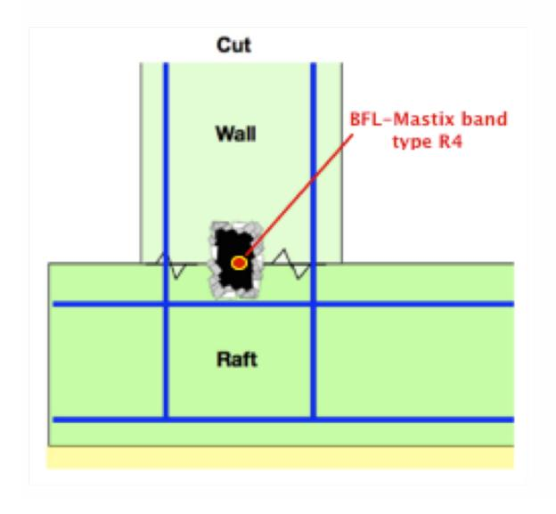
The BFL-Mastix waterstops consist of a soft and deformable core, covered with a limestons 4/8mm gravel, connecting afterwards with the cement in the concrete..
